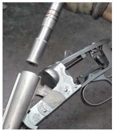
A worker checks chamber length to ready a gun for mandatory federal (and C.I.P.) inspection.
