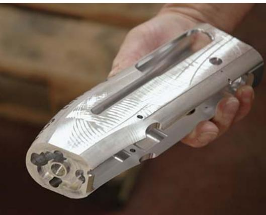
Receivers machined from lightweight alloy give Beretta autoloaders a lively feel and fast swing.
