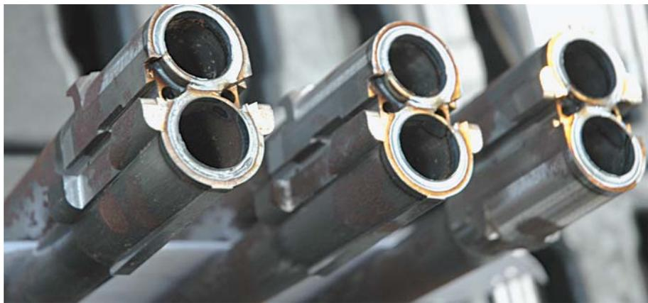
Barrels joined to monoblocks await finishing in a rack at Beretta 1, the main production plant.
