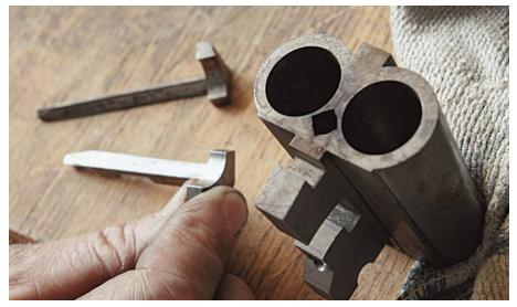
Massive lugs and triangular, full-length ejector rods give Fausti guns exceptional longevity.
