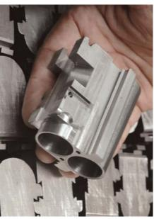
Fausti doubles incorporate forged monoblocks that are carefully machined and held to tight tolerances.
