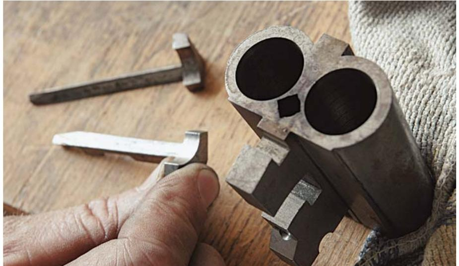
Massive lugs and triangular, full-length ejector rods give Fausti guns exceptional longevity.
