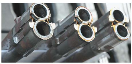
Barrels joined to monoblocks await finishing in a rack at Beretta 1, the main production plant.
