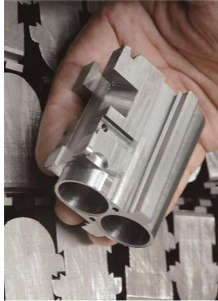
Fausti doubles incorporate forged monoblocks that are carefully machined and held to tight tolerances.
